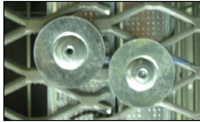
Figure 5: Example of mesh interlay seam, riveted
